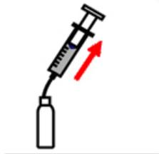
Assemble syringe and fill with RVS Master compound. This procedure will have to be repeated several times until all product is used
