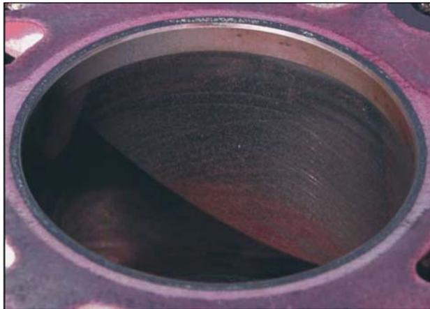
Figure 4-3: Digital recording of Ford Escort's engine block before treatment (honing marks on the cylinder surfaces are evident here)
