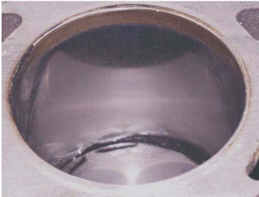
Figure 5-1: Digital recording of the Ford Escort's engine block following treatment (alterations to the surface are clearly visible)
